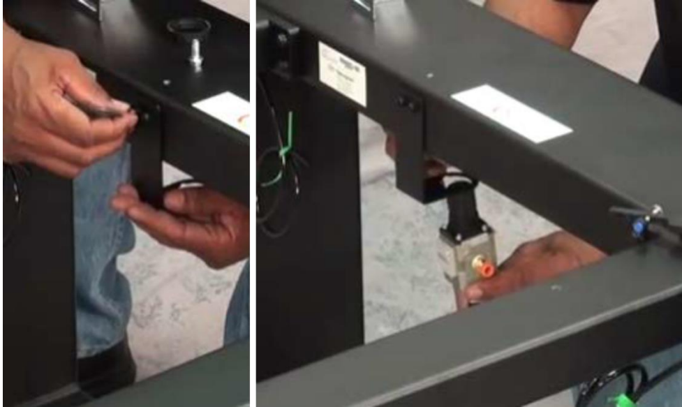
Figure 10: Air regulator filter (ARF) being installed on leg weldment.
