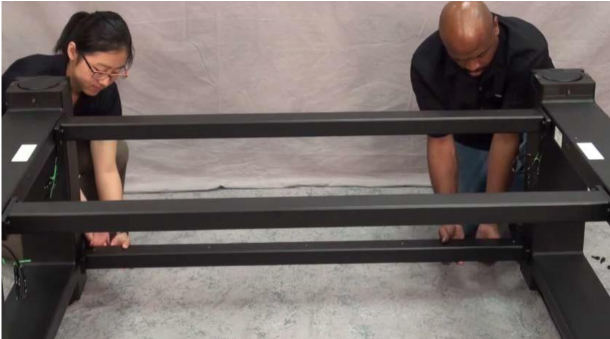
Figure 4: Connecting cross-braces to leg weldments.
